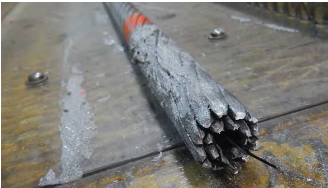
Figure 3-11. Celanese ACCR C 7 -TW Test Conductor after the Breaking Load Test
