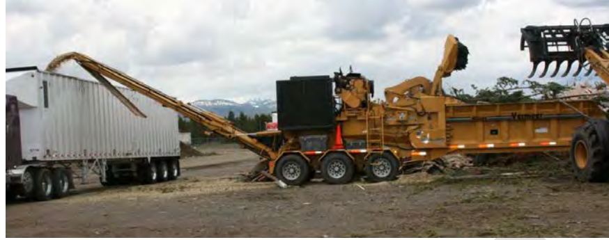
Figure 2-23. Vermeer HG6000 horizontal grinder conveys material into the top of a chip van. This is a “hot” loading operation with the system designed to keep the grinder operating at maximum efficiency.
