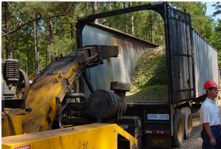
Figure 2-22. Mechanism of throwing material from chipper into back of chip van in Greenville, Alabama (Photo credit: Christopher Wright, INL, July 2010).
