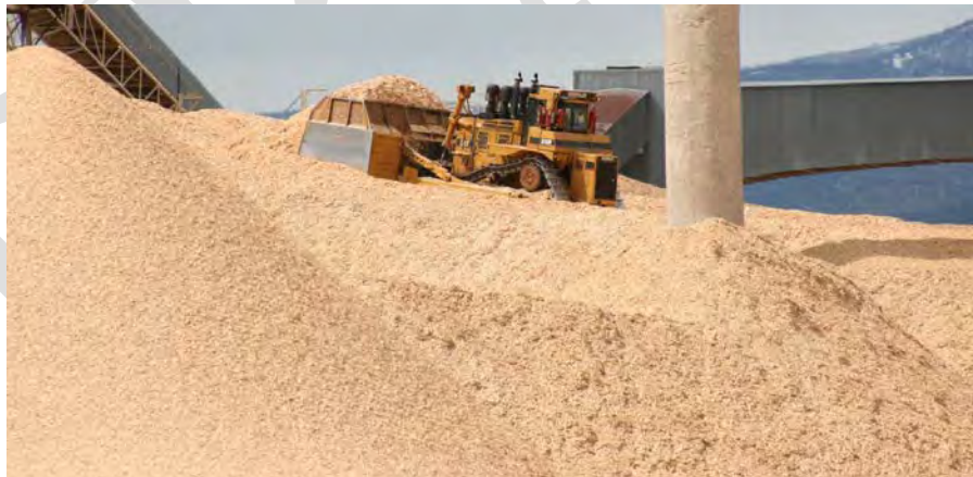
Figure 2-47. Tracked loader used to move chips during storage. The loader is equipped with an oversized bucket specialized for moving low-density, flowable materials (Photo credit: D. Brad Blackwelder, INL).
