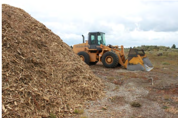
Figure 2-48. Case 629 front-end loader. Bucket has been modified by adding a screen to the top to increase payload (Photo credit: D. Brad Blackwelder, INL).
