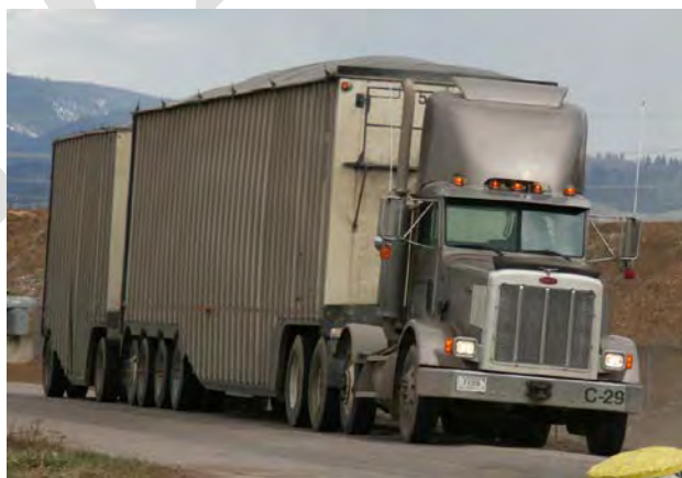
Figure 2-29. Possum belly chip van or trailer (Photo credit: D. Brad Blackwelder).
