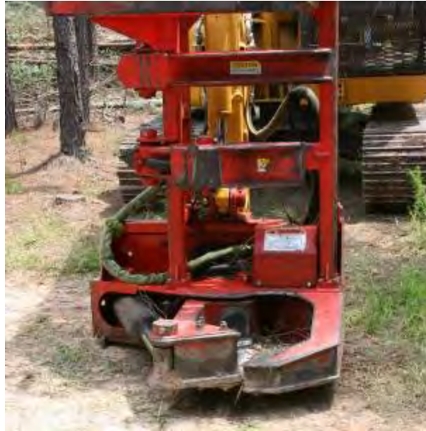
Figure 2-8. Rotary-head feller buncher. The upper arm holds the tree during felling, and the lower arm collects the tree after felling, forming a bunch (Photo credit: D. Brad Blackwelder, INL).
