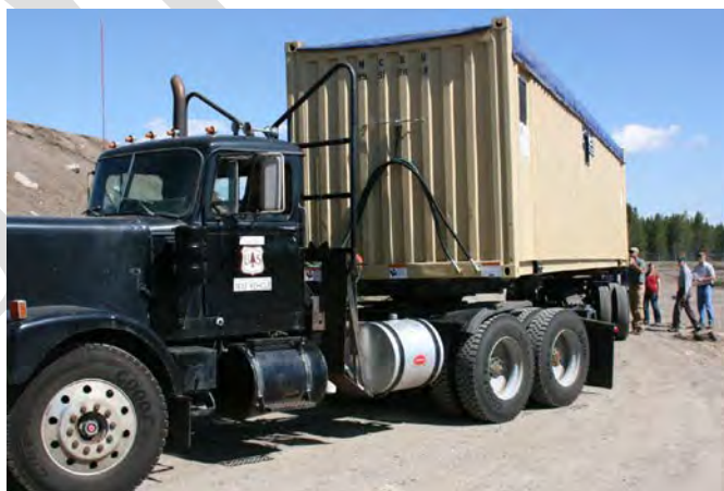
Figure 2-33. Stinger-steer chip van developed by San Dimas for accessing materials at remote landings (Photo credit: D. Brad Blackwelder, INL).
