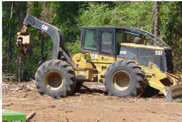
Figure 2-14. Wheeled grapple skidder with grapple head in Greenville, Alabama (Photo credit: Christopher Wright, INL, July 2010).
