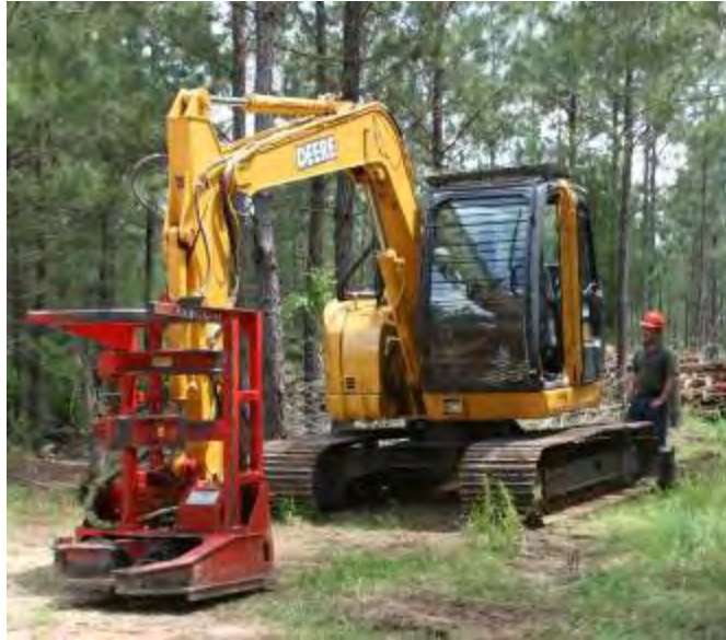
Figure 2-6. An accumulating head feller buncher mounted on a tracked excavator for a small diameter harvest study. Using smaller, less expensive, and more maneuverable equipment may improve efficiency when harvesting small trees (Photo credit: D. Brad Blackwelder, INL).
