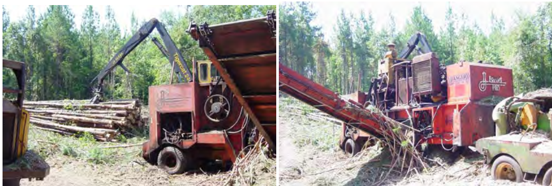
Figure 2-55. Flail shredder in Greenville, Alabama (Photo credit: Christopher Wright, INL, July 2010). The slash stream produced from delimbing and debarking trees is visible in the lower photograph.
