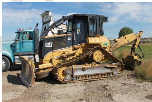
Figure 2-15. Caterpillar 527 tracked grapple skidder. This type of skidder is usually used on slopes from 15–30% grade (Photo credit: D. Brad Blackwelder, INL).
