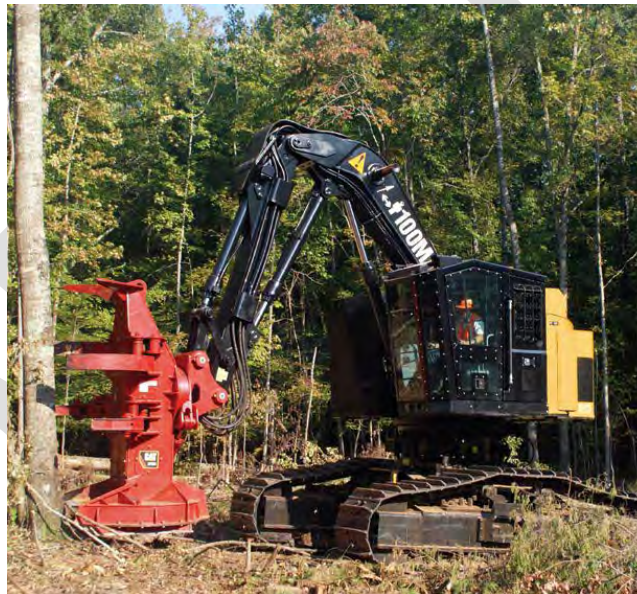
Figure 2-10. Typical tracked, swing-to-tree feller buncher (Cat 521) (Photo by Caterpillar 2010). Swing-to-tree tracked feller bunchers are often the only mechanized choice for felling operations on steep, erodible slopes. These machines often have self-leveling cabs that provide stability and reduce operator fatigue.
