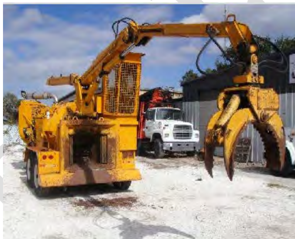
Figure 2-18. Chipper equipped with a boom and grapple (Photo credit: Wood Chippers & More 2011). The Base Case Conventional scenario uses a similar chipper design.
