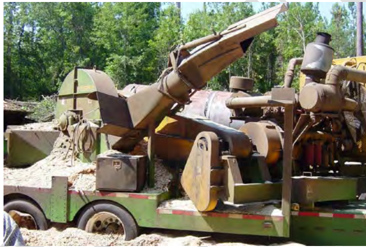
Figure 2-20. Disc chipper used to comminute whole trees (Photo credit: Christopher Wright, INL, July 2010).
