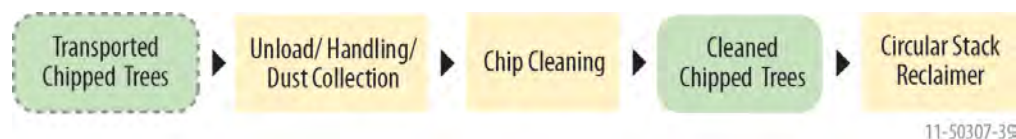
Figure 2-34. Receiving and Handling supply logistic processes and biomass format intermediates for the Base Case Conventional design. (Note: Green ovals represent biomass format intermediates and yellow rectangles represent processes modeled in this report)
