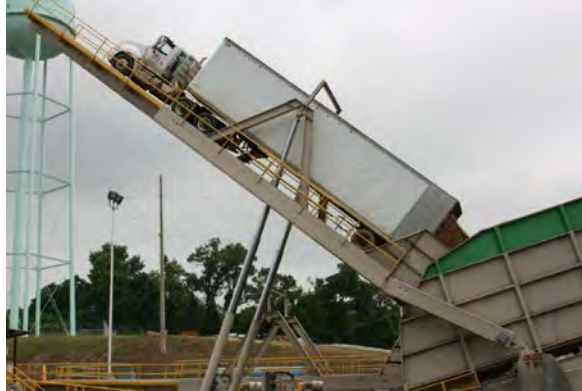
Figure 2-36. Whole-truck tipper unloading 120 yd 3 van loaded with comminuted wood to be further size-reduced and pelletized (Photo credit: D. Brad Blackwelder, INL).
