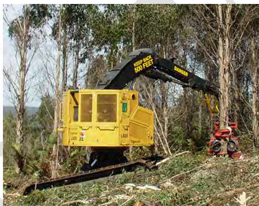
Figure 2-12. Tigercat LH830C harvester suitable for CTL operations on steep terrain (photo from Tigercat (2010)).
