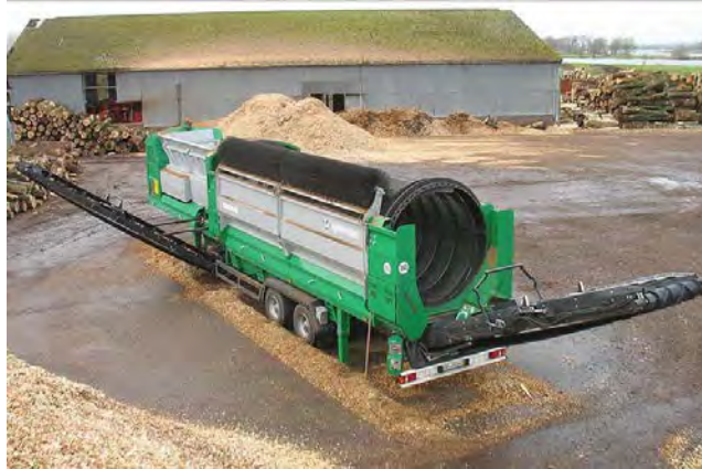
Figure 2-57. Magnum Komptech trommel, used to separate chips (Photo from Wikipedia.com 2010)
