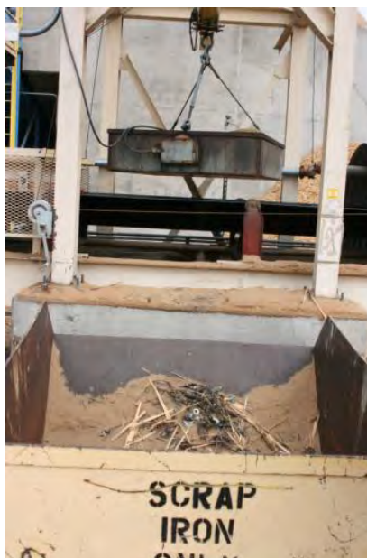
Figure 2-37. Magnet over a conveyor at a paper mill (Photo credit: D. Blackwelder, INL).
