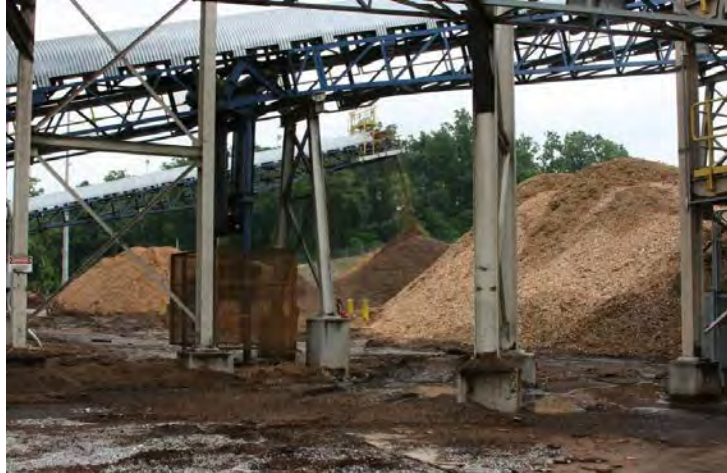
Figure 2-46. Woodchips stored outdoors at a pellet mill in Alabama are vulnerable to moisture infiltration. In this photo, puddles of water near the chips are clearly visible (Photo credit: D. Brad Blackwelder, INL).
