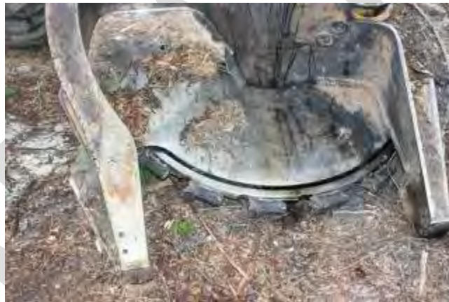
Figure 2-7. Rotary-head feller buncher cutting blade. The upper metal disc is stationary, while the lower toothed disc rotates and cuts the tree. Teeth are bolted on individually and replaced as needed (Photo credit: D. Brad Blackwelder, INL).
