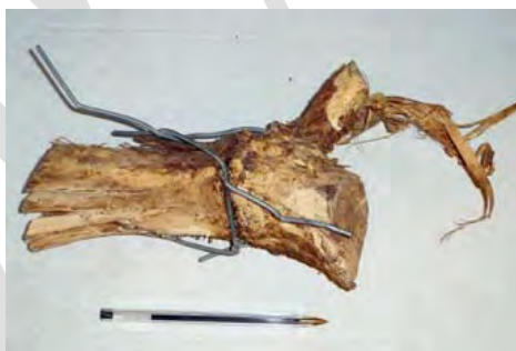
Figure 2-38. Entrained metal fragments can be of various sizes. The metal can potentially damage equipment and also increases the risk for spontaneous combustion (Photo credit: Regensw Sustainable Energy Agency 2008).
