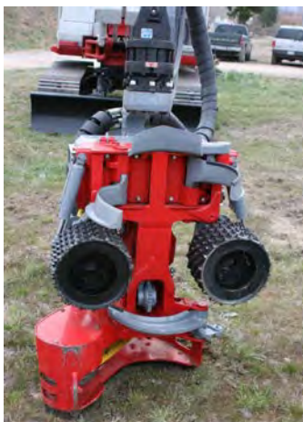
Figure 2-11. Processing head mounted on a tracked, swing-to-tree, primary mover for delimbing and bucking at the stump in a CTL harvest system. This type of head can also be used at the landing to process trees (Photo credit: D. Brad Blackwelder).
