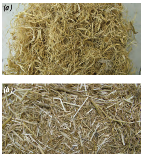
Figure 2-29. Corn stover (a) and switchgrass (b) ground with a tub grinder through a 1.5-in. screen. The corn stover picture (a) shows the fibrous mat that remains in the grinding chamber at the end of the grinding process. All of the switchgrass (b) is discharged from the system, leaving no fraction in the grinding chamber.
