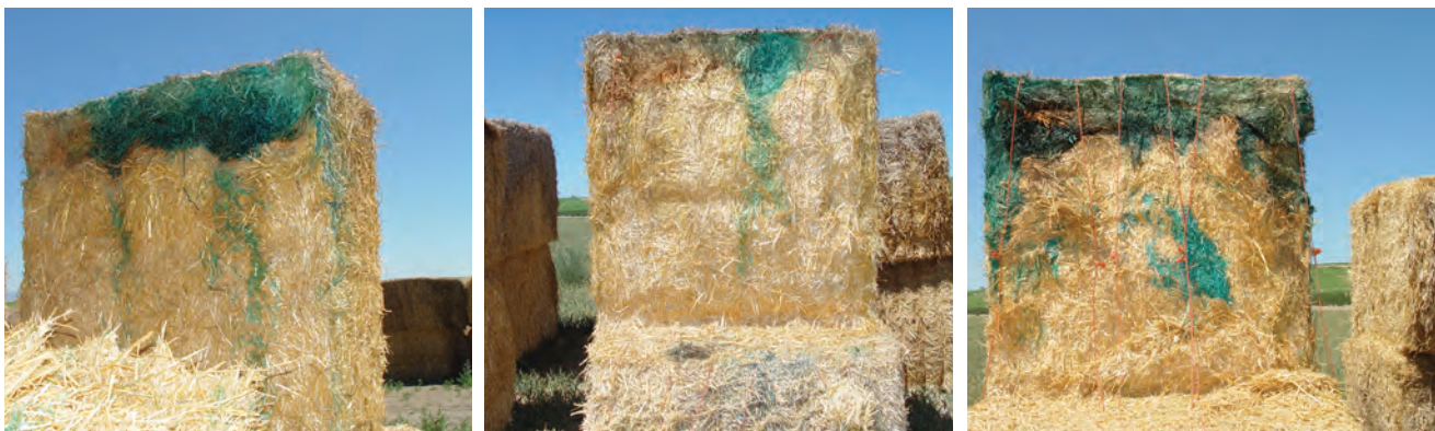
Figure 2-13. Large square wheat straw bales from the top of a stack stored field-side in Idaho. Note that water channeling, shown by the dark blue food dye, extends well past the region of damaged straw (dark brown straw) that is visible.
