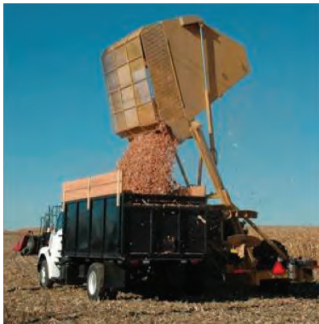
Figure 3-11. With a truck positioned beside the cob wagon, the harvest operation is temporarily stopped to dump the cob wagon bin. Vermeer Corp. CCX770 Cob Harvester.
