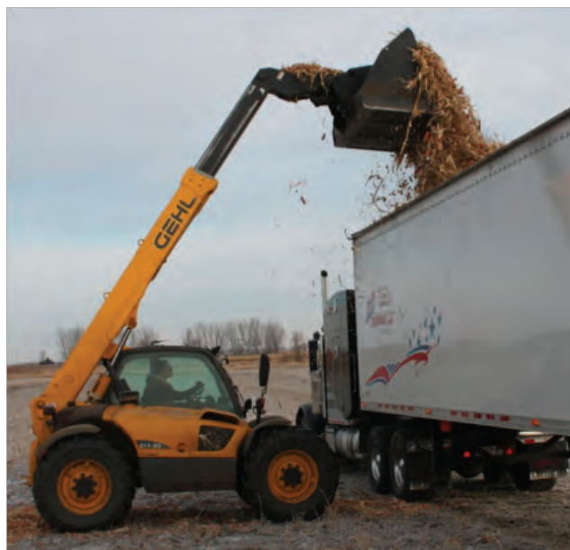
Figure 3-28. Telehandler loader used to load corn cobs for transport to the biomass depot.
