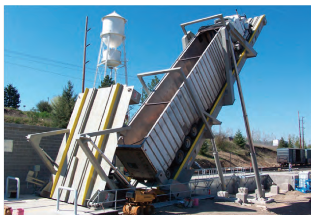
Figure 3-34. Receiving processes within the Pioneer Uniform design: Phelps drive-through truck tipper.
