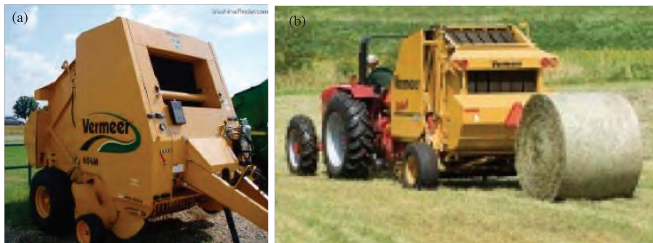
Figure 3-7. Round baler: (a) Vermeer 604 Super M Large Round 5.5x4-ft round baler (b) pulled by a 115 hp mechanical front-wheel-drive tractor with a round bale that has just been discharged from the baler.
