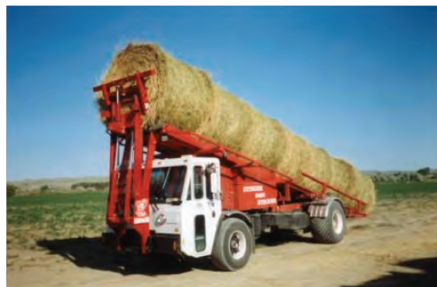
Figure 3-8. Stinger Stacker 5500 loaded with round bales.
