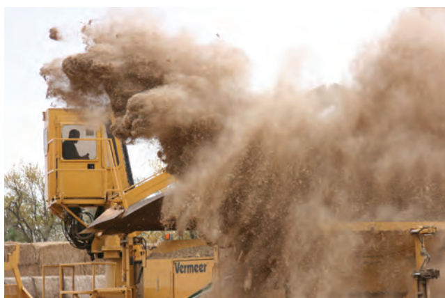
Figure 2-34. Dust emissions as corn stover bales are preprocessed in a tub grinder.
