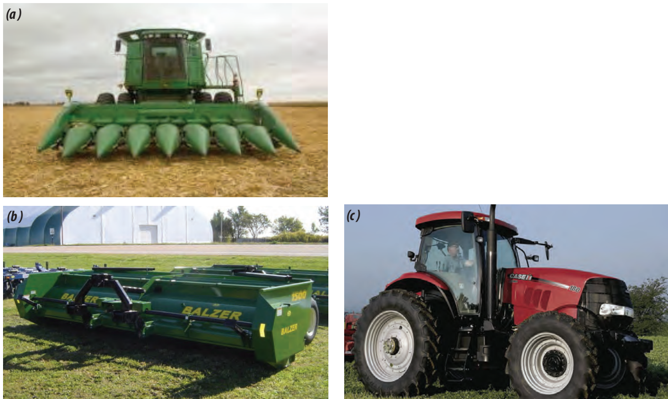
Figure 2-5. Conventional Bale–Stover harvest equipment (combine with grain harvest header [a] and shredder/windrower [b] that is pulled by a tractor) is functionally different than Switchgrass harvest equipment (self-propelled windrower [c]).
