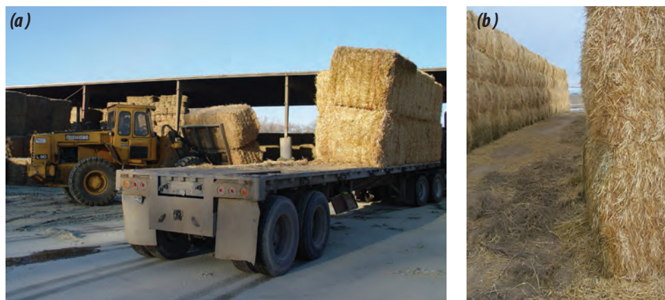
Figure 2-26. Receiving and queuing processes within the Conventional Bale receiving and preprocessing unit operation: (a) Bale handling and truck unloading and (b) lane separating two stacks of 4×4×8-ft bales in a bale yard.
