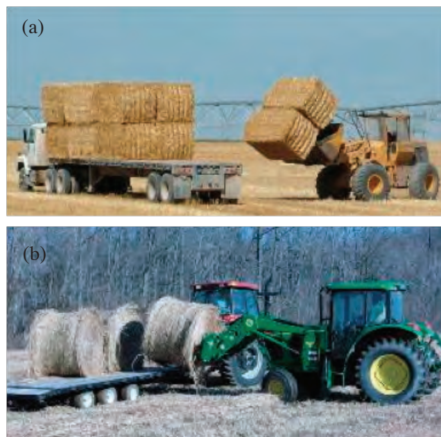
Figure 3-6. Biomass bales being loaded onto haul trailers: (a) large square bales can be handled two at a time, while (b) round bales can only be handled one at a time for proper orientation of the trailer.
