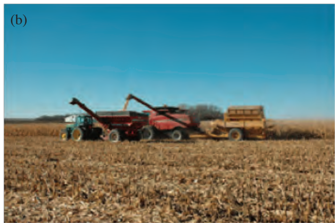
Figure 3-9. Harvesting both grain and cobs; (a) CNH combine pulling a Vermeer cob wagon in a corn field near Holloway, Minn., during the Chippewa Valley Ethanol harvesting demonstration Oct. 28, 2008;h (b) John Deere combine pulling a Redekop Manufacturing cob wagon (Source: Redekop Manufacturing)
