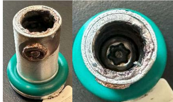
Figure 4. Side and top view of a damaged CCS connector DC pin. Photos by NLR
