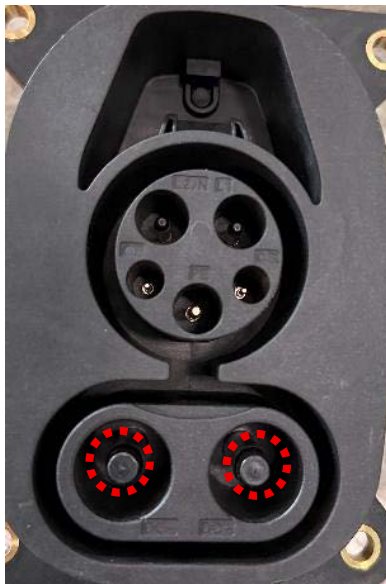
Figure 1. CCS charging inlet with the insulated DC pin end caps attached. Photo by NLR
