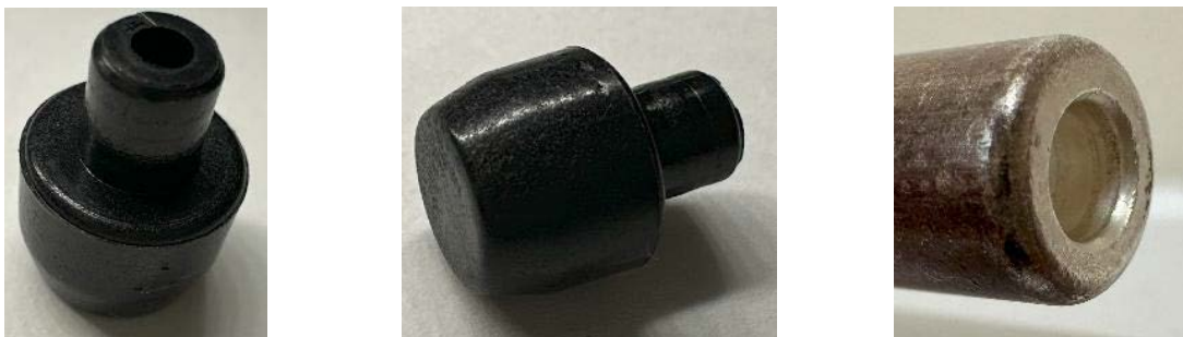
Figure 5. Insulated end cap with its associated pin structure. Photos by NLR
