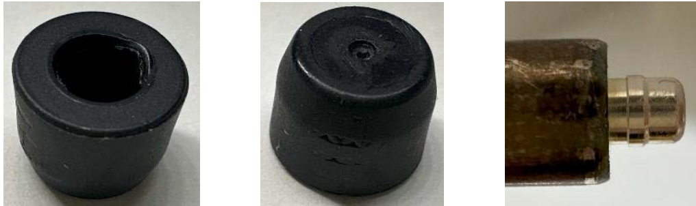
Figure 6. Insulated end cap with its associated pin structure. Photos by NLR
