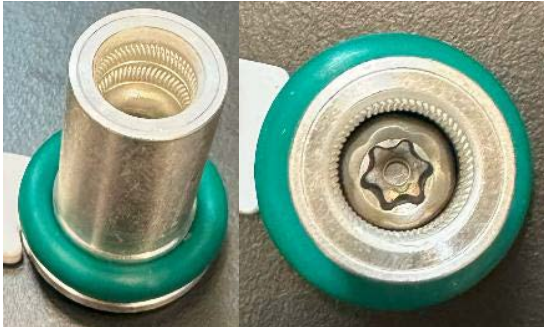
Figure 3. Side and top view of a CCS connector DC pin. Photos by NLR
