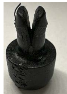
Figure 24. Type B insulated end cap for Manufacturer C. Photo by NLR
