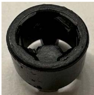
Figure 23. Type A insulated end cap for Manufacturer C. Photo by NLR
