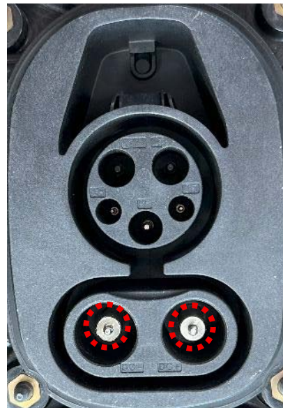
Figure 2. CCS charging inlet with the insulated DC pin end caps detached. Photo by NLR
