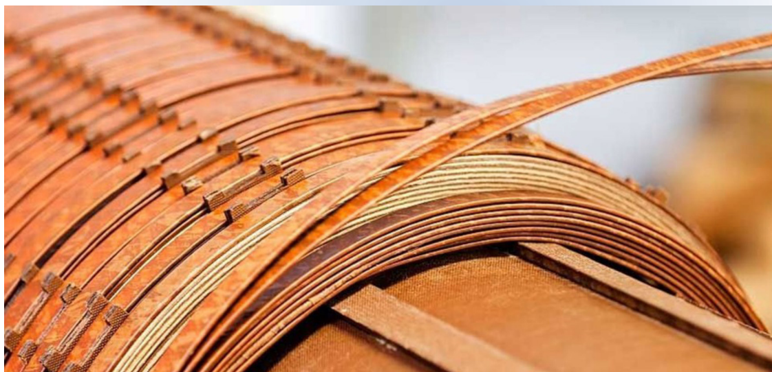
Figure 1. Insulation wrapped conductor being wound onto a transformer core.
