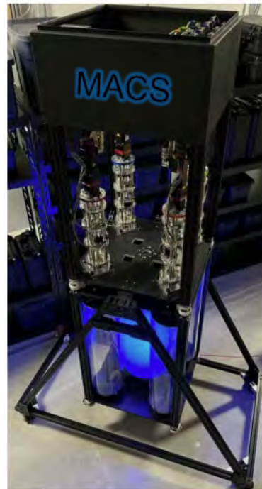
MACS Hardware (non-nuclear surrogate for MARVEL controls)
