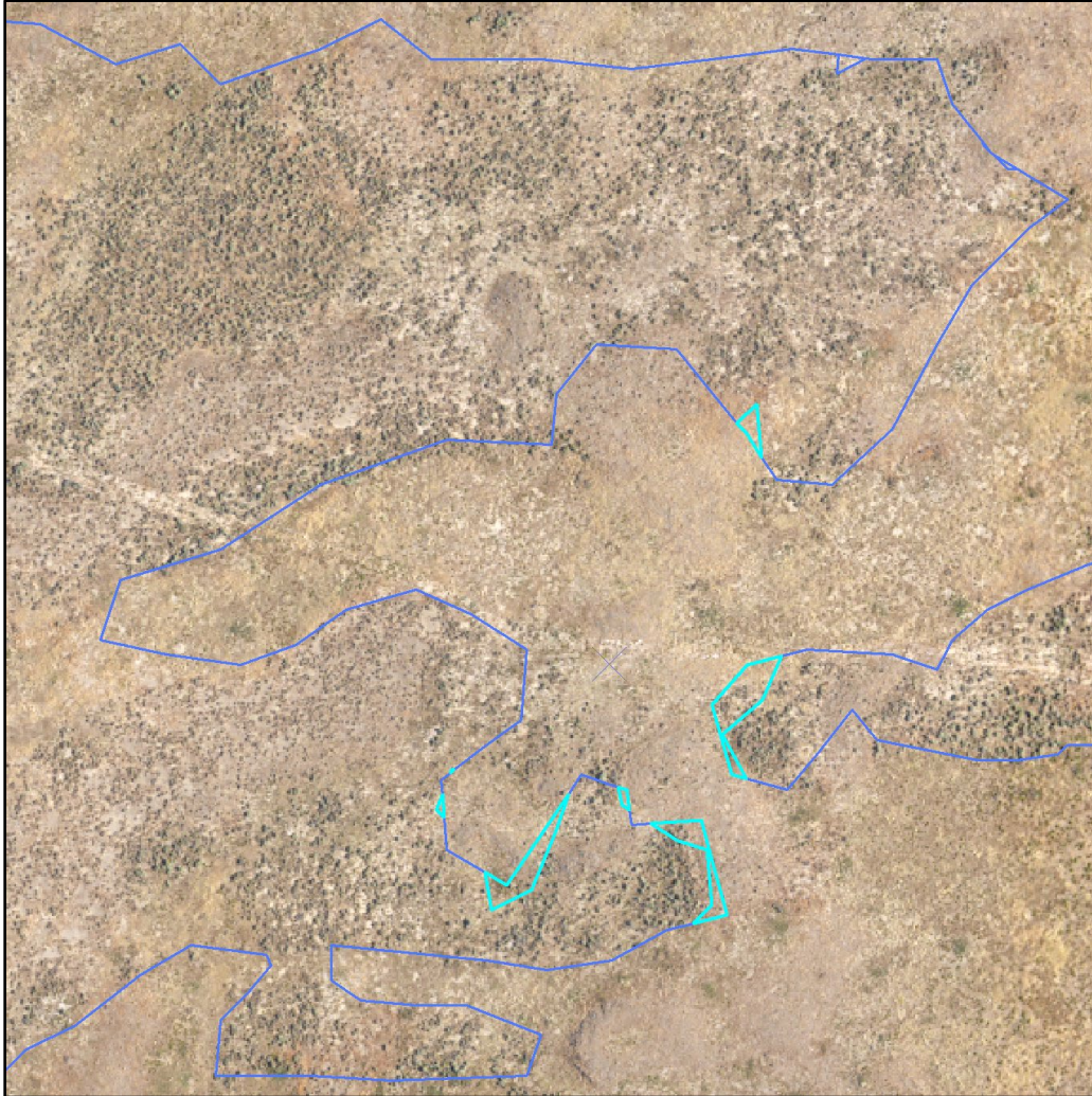
Figure 3. The light blue highlighted polygons are all part of one polygon that was clipped to the mapped burned area. The darker blue polygons show unburned patches of sagebrush that were mapped following the 2019 Sheep Fire. The three smallest light blue polygons were well below the mapping scale and were removed from the dataset.
