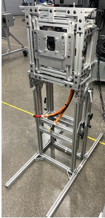
Figure 4. View of the inlet force evaluation fixture
