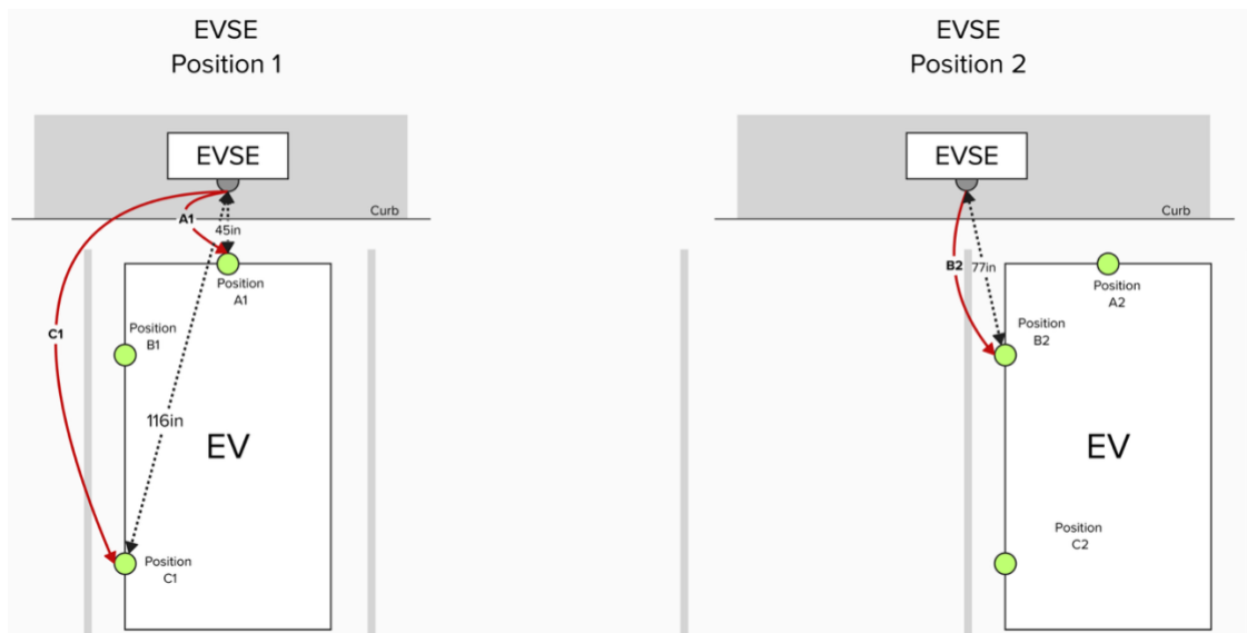
Figure 6. Graphical description of the three different positions used in the evaluations
