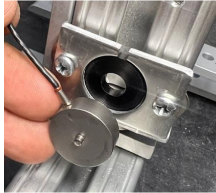
Figure D-4. Neoprene round spring behind the sensor, allowing for a small amount of flexibility
