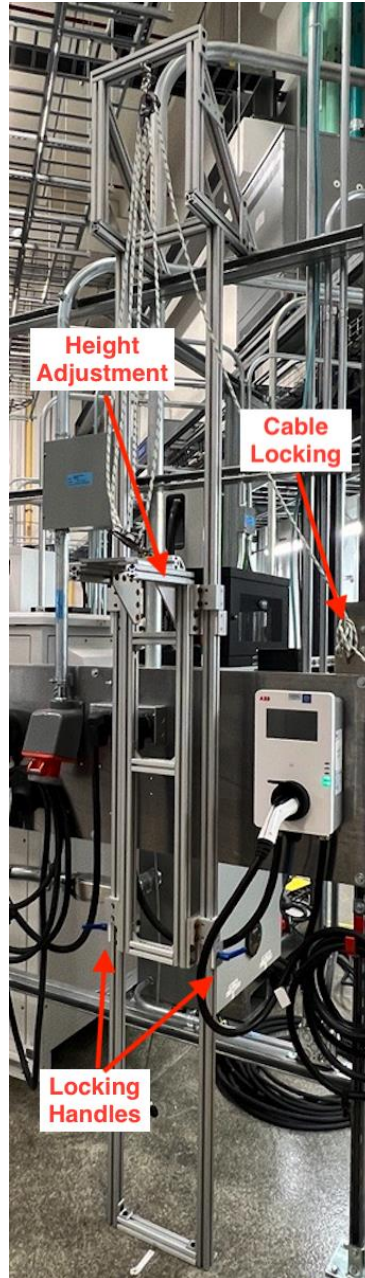
Figure B-1. View of the EVSE fixture for holding the EVSE cable/connector assembly
