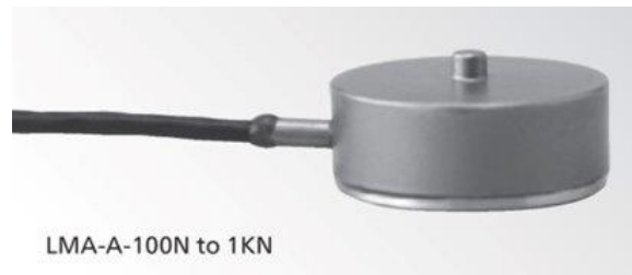
Figure C-1. Image of one Kyowa 1-kN load cell
