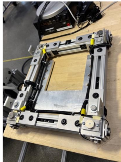
Figure D-6. Final view of the inner frame wired up with all 12 load cells in groups of 3 at each corner, with the metal plate ready to have an EV inlet mounted
