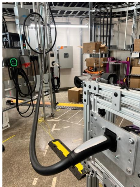
Figure 8. Mated connector during NACS-to-NACS evaluation setup in the lab
