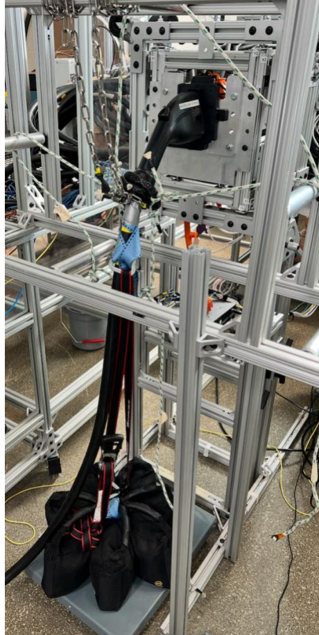
Figure 12. Image of the 750-N evaluation setup, showing the principal weight resting on a scale.
