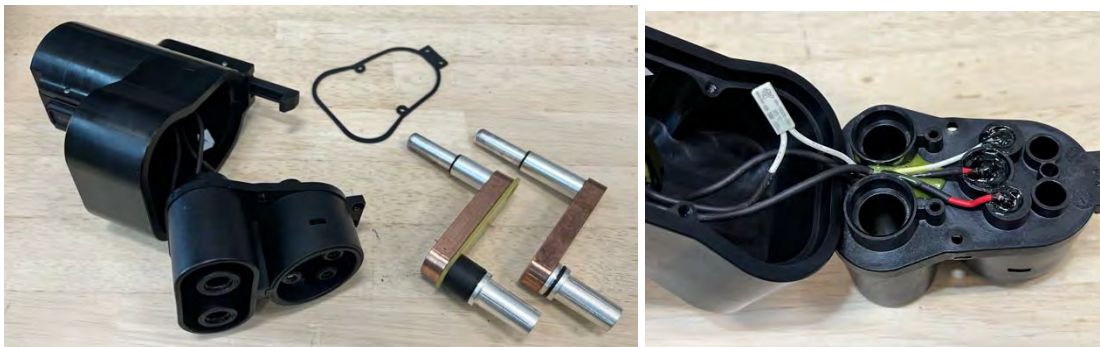
Figure 2. A disassembled J3400-to-CCS adapter
