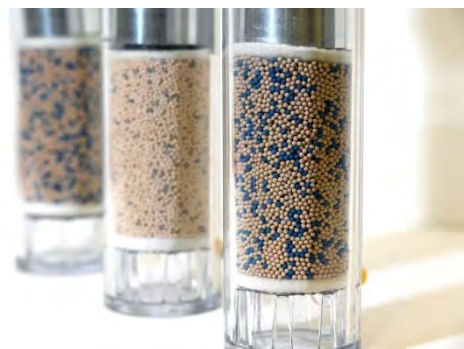
Figure 4-6. Atmospheric moisture collection columns.
