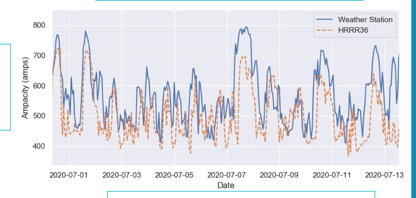
Plot of HRRR 36 Model Versus Weather Based Ampacity
