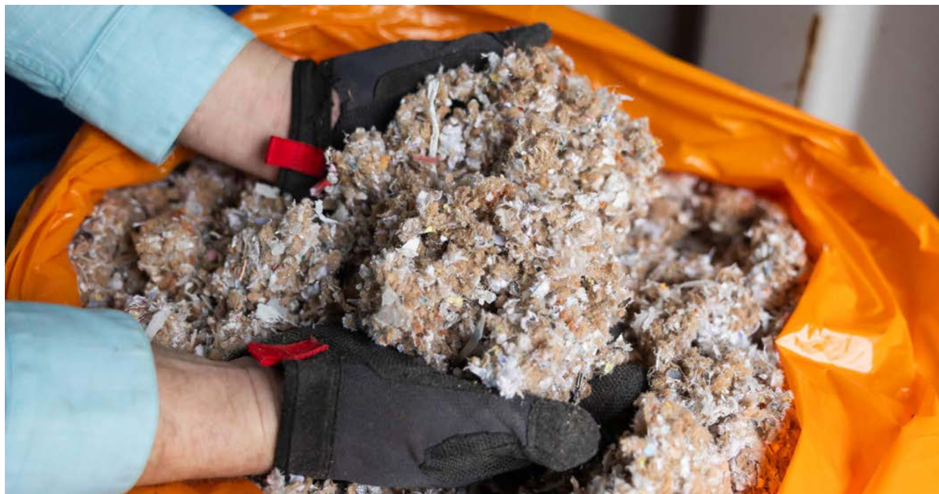
ReNuFiber's thermal insulation is made from non-recyclable plastics, textiles and wood.
