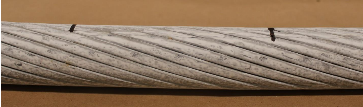
Figure 4: Very light flattening shown on a 150 lb/in sample with marks indicating the span where the bottom platen made contact
