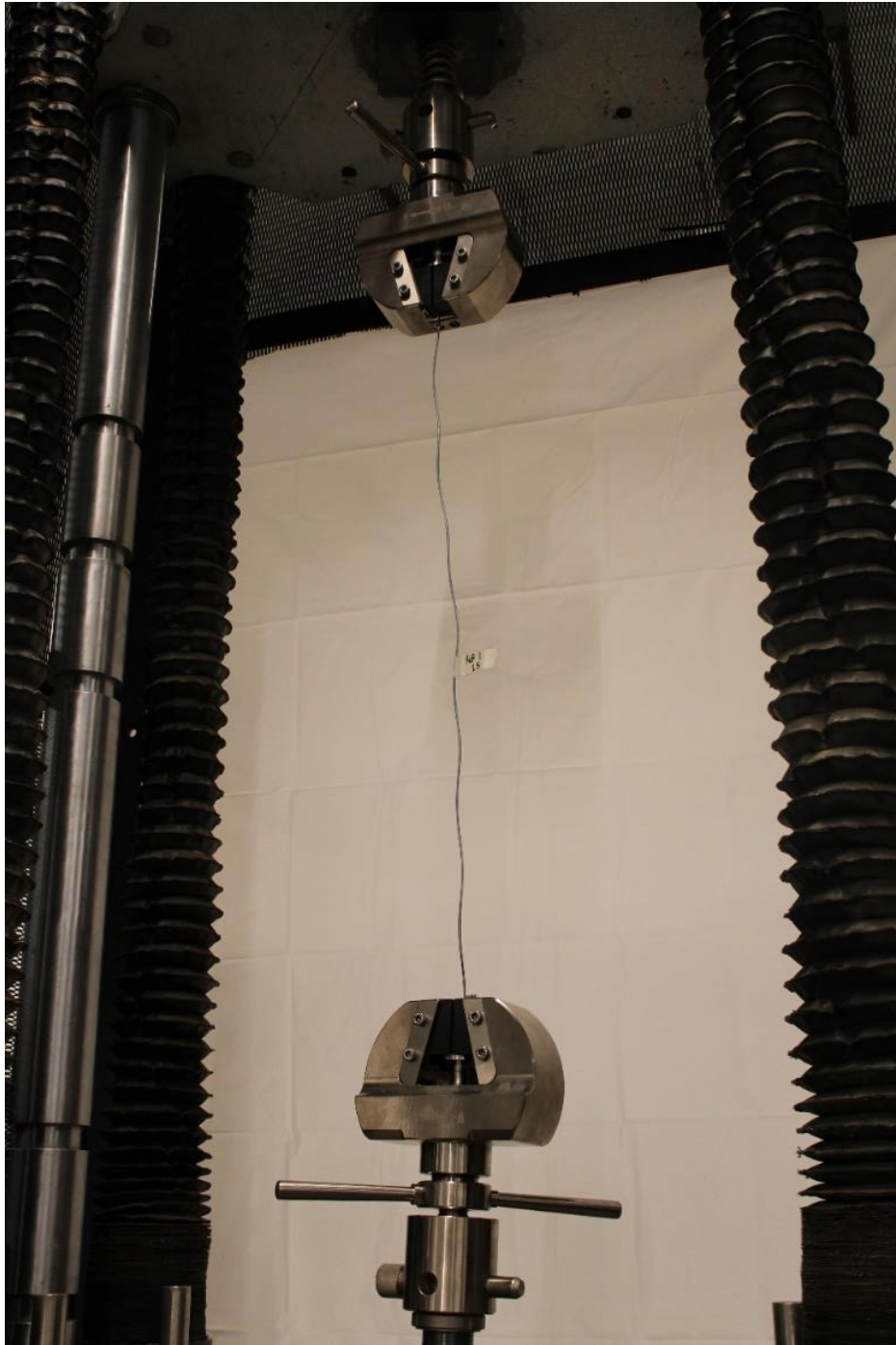
Figure 3: Sample installed in UTM before testing
