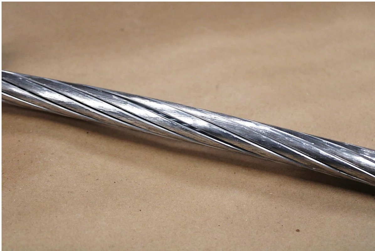
Figure 5: Example of marks on inner aluminum strands from upper layer
