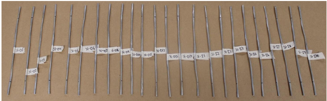
Figure 1: Test Samples Before UTS Testing
