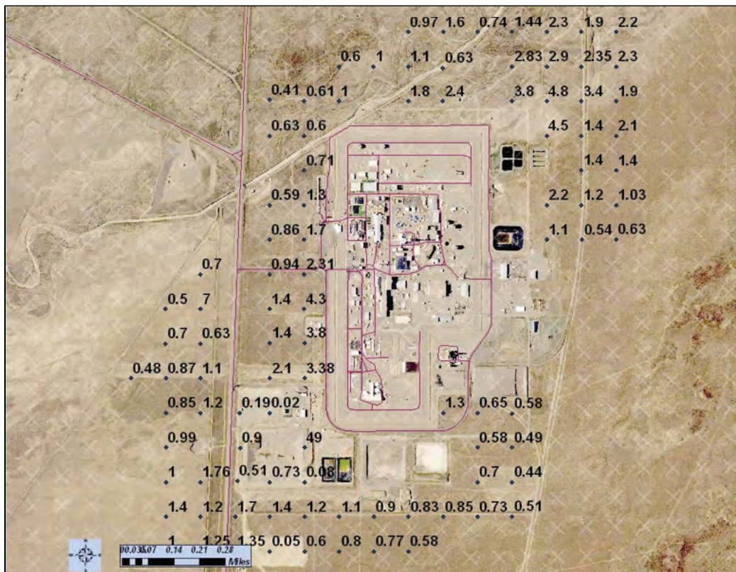
Figure E-4. 2007 In Situ Gamma Scan Results (pCi/g) for ^{137}\text{Cs} at INTEC.
