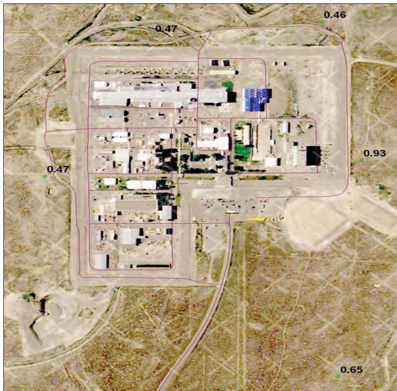
Figure E-6. 2007 In Situ Gamma Scan Results (pCi/g) for ^{137}\text{Cs} at NRF.
