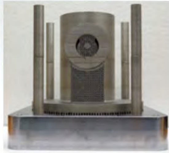
Figure 1b. A 316L SS section of a valve body was produced via LPB-AM.
