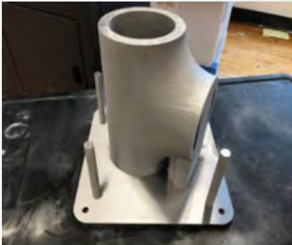
Figure 1a. A 316L SS Pipe Tee fitting is being produced via LPB-AM.
