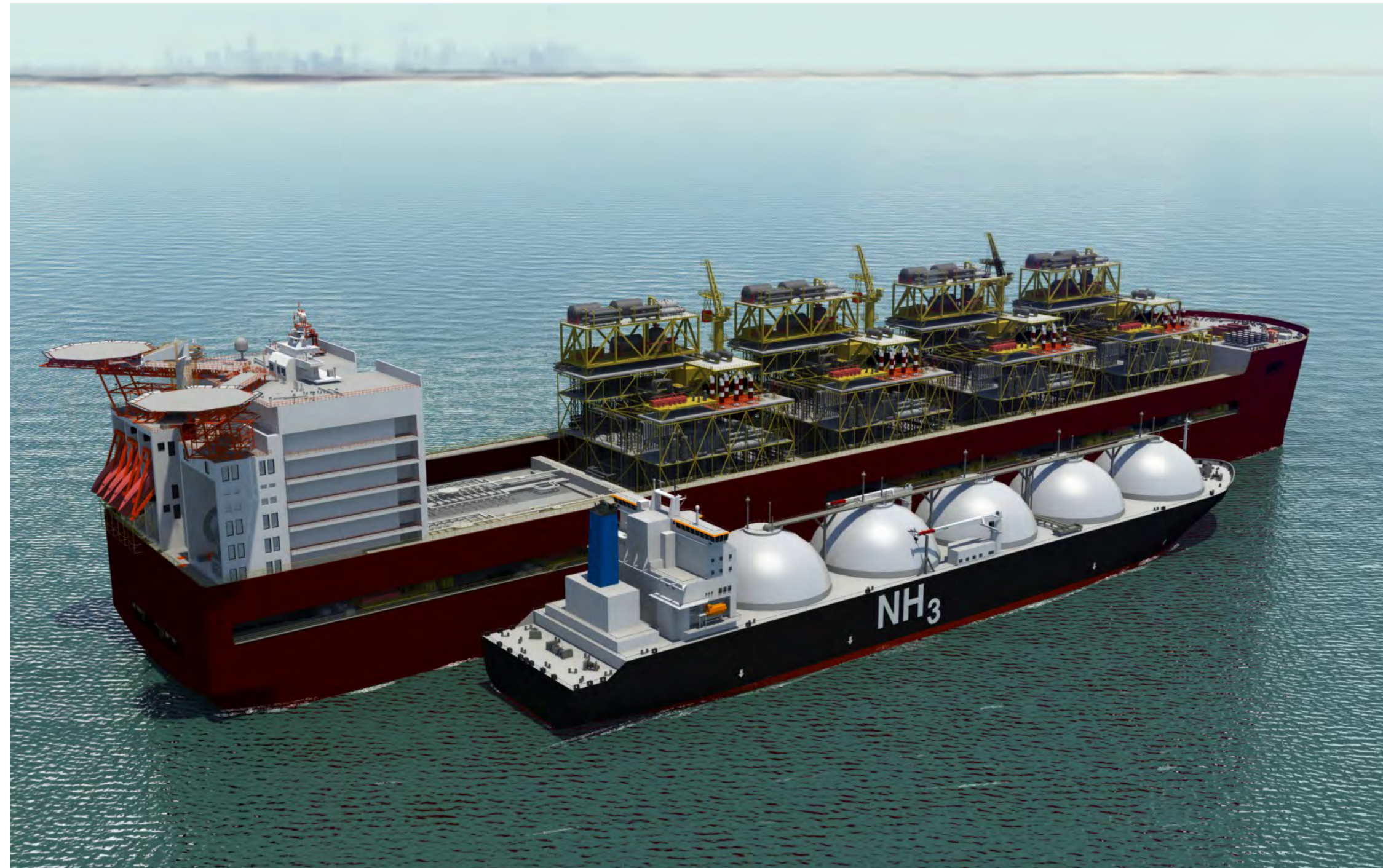
Ammonia bunker offloading ammonia from production platform
