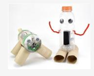
When you turn the battery pack on, it completes an electrical circuit with the motor. This causes electricity to flow in a loop from the batteries through the motor, making the motor spin. Because the motor has a weight attached to its spinning shaft, it wobbles and makes the entire robot's body vibrate, causing it to move. This is the same concept that makes video game controllers and cellphones buzz—they have tiny vibrating motors inside them!
