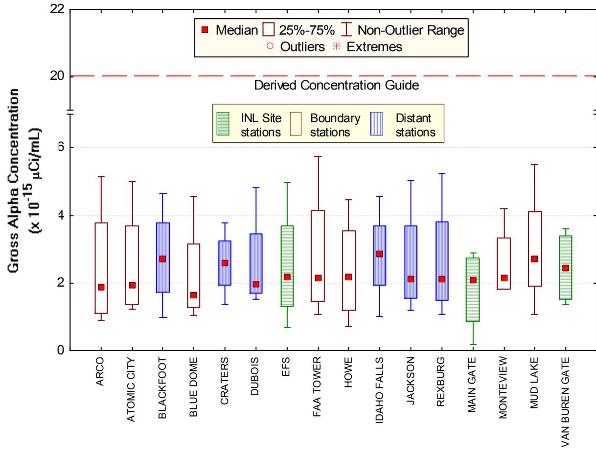
**Figure 6. September 2006 gross alpha concentrations in air at ESER Program INL, Boundary, and Distant locations. Number of samples (N) = 4 at each location.**
