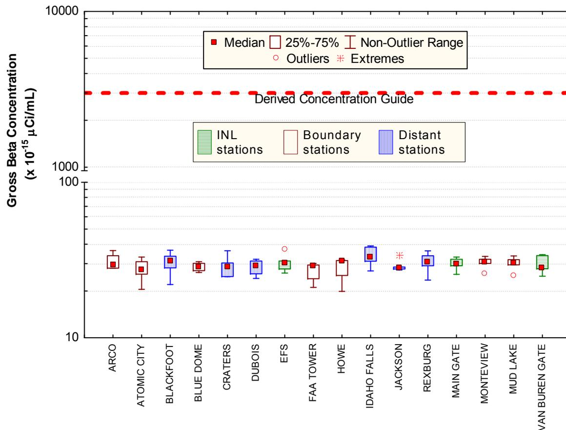
**Figure 9.** August 2006 gross beta concentrations in air at ESER Program INL, Boundary, and Distant locations. Number of samples (N) = 5 at each location except Arco and Blue Dome where N = 4.
